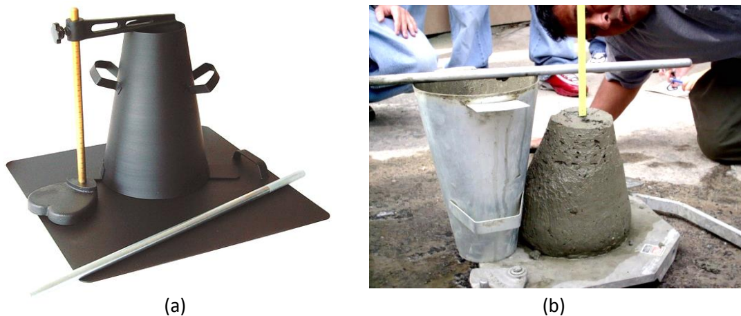
Figure 44: (a) Test Apparatus – Abrams cone or slump cone (b) Concrete Slump
