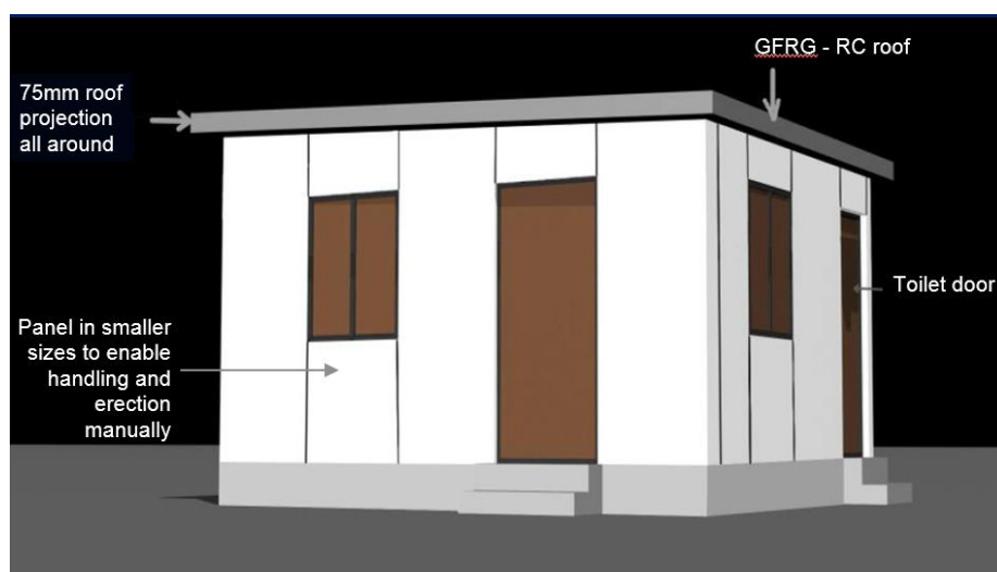
Figure A14.3 Housing suitable for rural poor in the suburban parts of rural areas
