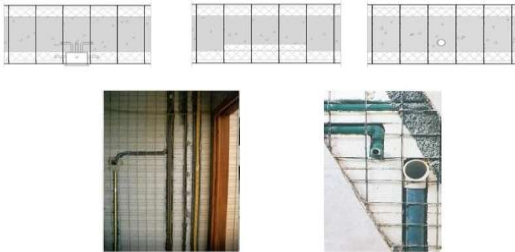
Fig. 53 Ducts embedded into concrete and/or insulation strips, either pouring concrete or afterwards in the insulation (cut or malt)
