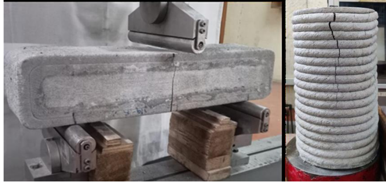
Fig. 14 Printed beam and cylinder with grout
