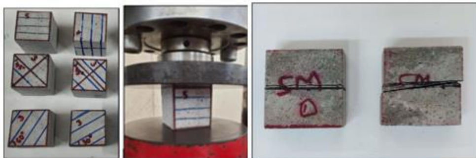
Fig. 18 Extracted element – Cubes with different orientations and bond strength
