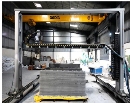
Fig. 3 Printing setup Gantry based – Off-site
