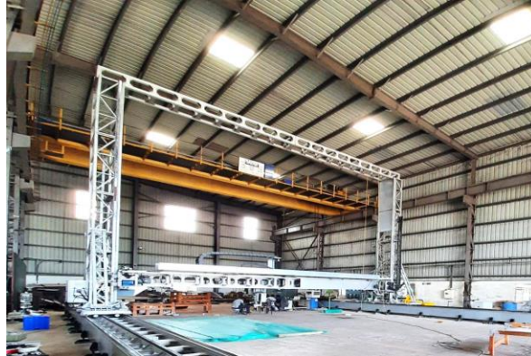
Fig. 4 Printing setup Gantry based – On-site
