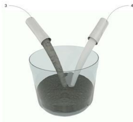
JOINTING COMPOUND PREPARATION MIXING RATIO A / B = 3/1
