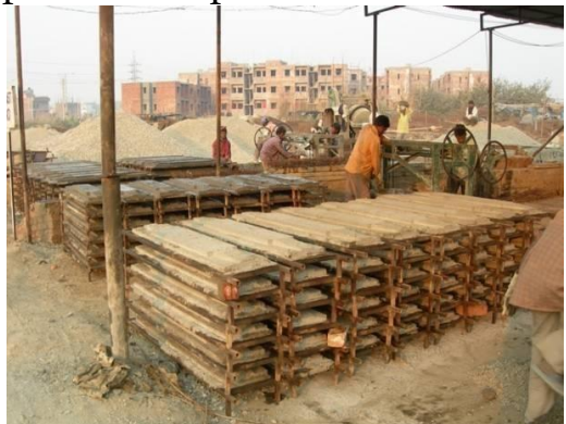
Fig.29 Casted planks on pellets stacked for initial strength
