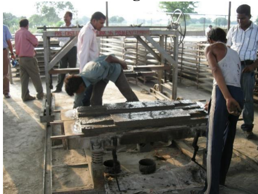
Fig.27 Ready casted twin planks over pellets
