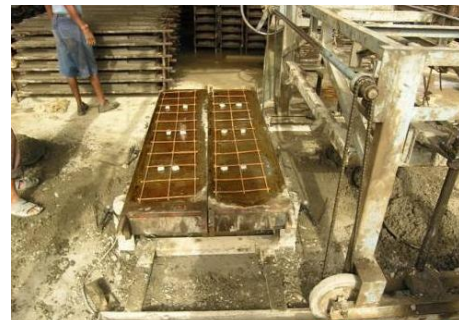
Fig.24 Placing twin plank reinforcement
