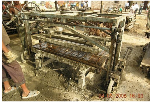
Fig.25 Placing mould over reinforcement cage
