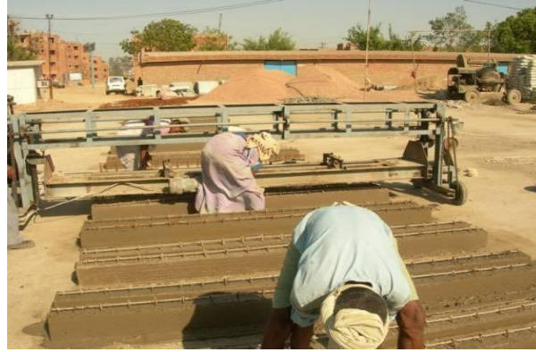
Fig.11 – Precasting of joists with egg laying machine
