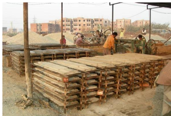
Fig.10 – Casted planks on pellets stacked for initial strength
