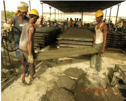
Fig.28 Lifting casted plank with pellet
