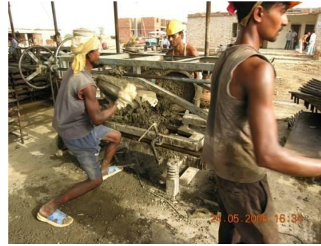
Fig.26 Pouring of concrete in mould
