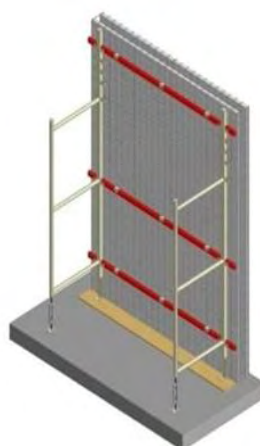
Fig. 26 Strut Fig. 27 Stanchion and strut for stanchion to create guardrail, board to align panels
