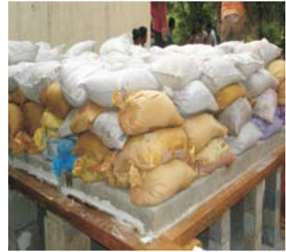
Load test on the precast panel
