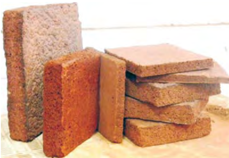
Fig.2 Light weight foamed slabs and tiles s made from red mud
