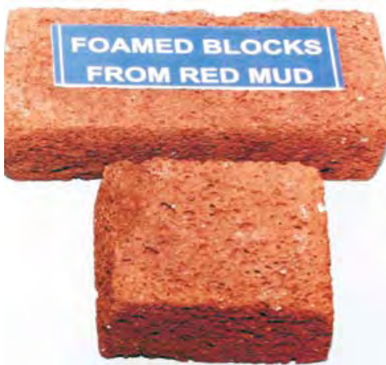
Fig.1 Light weight foamed bricks from red mud
