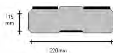
Steel Plates: 50mm x 240mm x 10mm Figure 7: Test Sample- Block with Bed Plates
